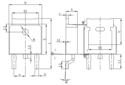
The outline from different package houses may have slight differences. So the outline above is just schematic. The dimensions are controlled per specifications.
